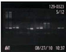
OmniDOC Software – complimentary basic image analysis software supplied with all omniDOC systems for molecular weight or size determination in 1-D gels
