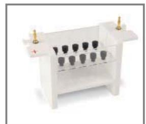
The omniPAGE Mini capillary tube gel insert may be used for IEF of up to 10 capillary tube gels in as little as 3.5 hours (Pg 60)
