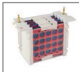
The omniPAGE Mini blotting insert is available in traditional wire electrode format or with rapid high-intensity plate electrodes (Pg 79) to transfer up to 4 and 2 gels respectively
