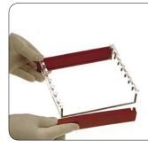
Casting dams allow gels to be rapidly cast externally while the unit is in use for gel running
