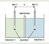
values, this layer will have a low hydrogen concentration. However, at low pH values a large number of H+ ions diffuse in the layer. By measuring the generated electrical potential (E) in the layer the corresponding pH can be computed.
