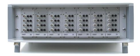
pH: 0...14 pH mV: ±2000 mV lon: 0...100 g/l 0...2000 mS/cm Conductivity: TDS: 0...100 g/lDissolved oxygen:  $0...60 \, \text{mg/l}$ Temperature: -5...+105°C
