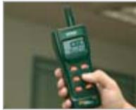
Measure CO<sub>2</sub> level in office buildings to insure proper ventilation.
