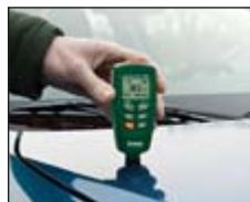
Measuring the thickness of automotive paint
