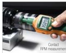
Contact RPM measurement
