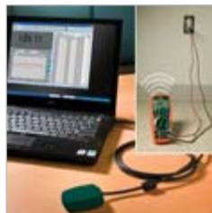
Meter features include continuous wireless data streaming to a PC in real time, drop-proof tested to 6.5ft (2m), and waterproof design (IP67).
