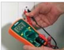
Displays AC Voltage of an outlet receptacle
