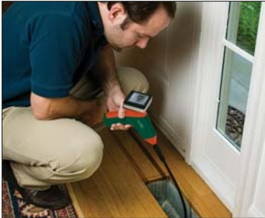
**3.5" Color Detachable Wireless LCD Monitor can be viewed from a remote location up to 32ft (10m) from measurement point**
