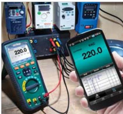
View key electrical readings taken by the GX900 at a safe distance from your Android device. Power up equipment from remote switches or use your Android to show readings to a customer/manager. Download the Extech GX900 ExView™ App at [play.google.com](http://play.google.com).
