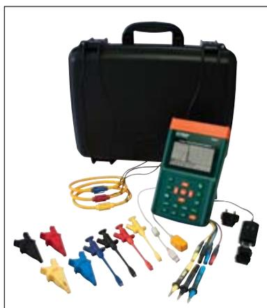
Includes (3) flexible current clamps, (4) voltage leads with alligator clips and retractable plunger clips, 8 AA batteries, universal AC adaptor, software, USB interface cable, and case; 1 year warranty.
