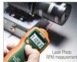
Laser Photo RPM measurement
