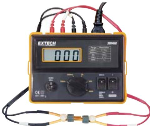
**Portable Milliohm meter provides resolution to 0.1mΩ**
