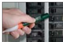
Non-contact InfraRed Temperature measurement
