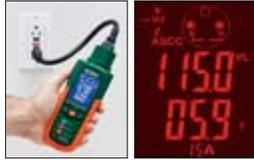
Both models Test 3-wire standard & GFCI receptacles. Display turns red when a problem is detected. CT80 also has AFCI function.
